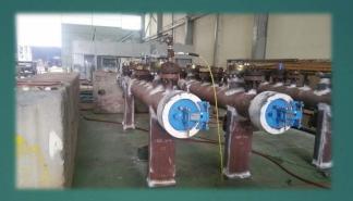
Pig Launcher & Receiver:
