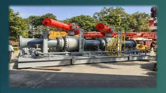
HIPPS Skid: 30" ESD Valves +LogicSolverPanelInstrumentation+Instrumentation+Skid.DesignPressure100Bar(g);Size:30"600#;38mmThk.MaterialCarbonCarbonSteelASTMA105/A106A672.NACEMR0103/MR0175;StressReliving(PWHT).HighSourServiceHydrocarbonHuid.
